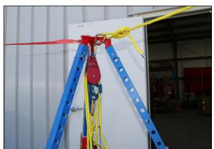
Attach your high angle rescue systems to the three anchor holes under the tripod head.
