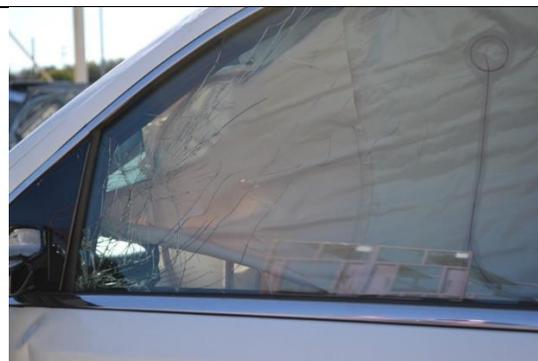
Laminated side glass cracks but stays in place. Note the large, persistent side restraint curtain that blocks the view of interior. These windows are very, very hard to remove!
