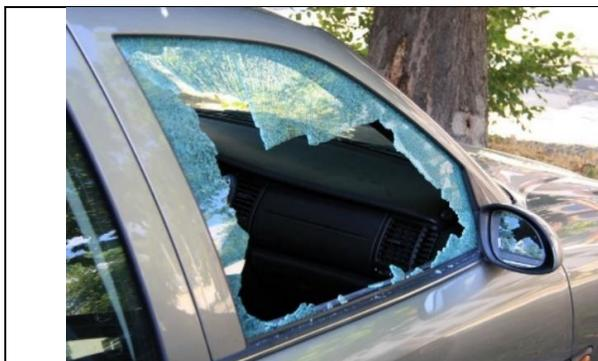
Standard broken tempered glass side window. Note the complete fracture and glass pebbles. These windows are very easy to remove.
