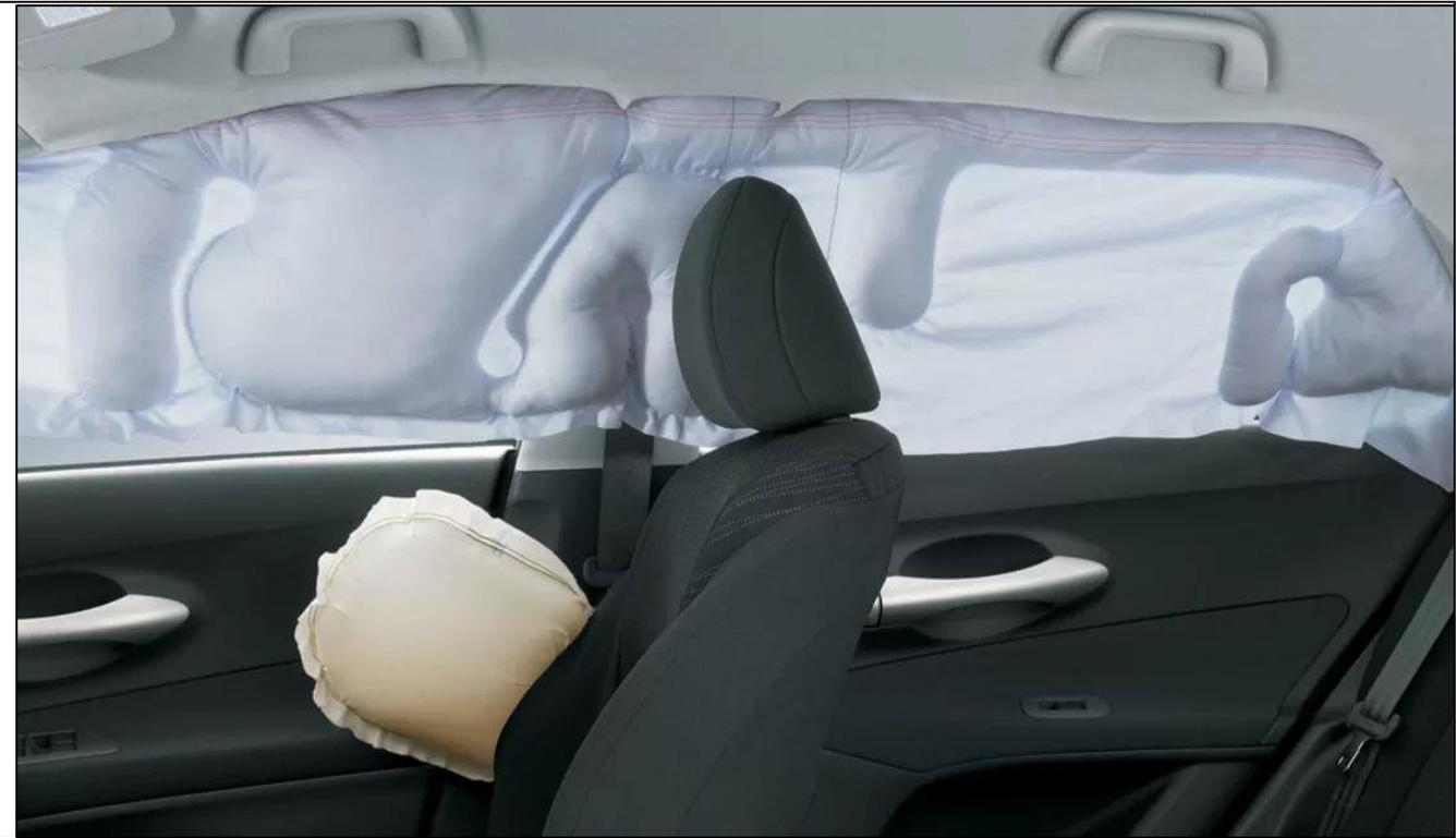
FMVSS 226 requires side airbags and Anti-Ejection curtains to help prevent occupant ejection during a rollover. They stay in place after the accident and will block the view of occupants/victims. They will need to be cut free. Using axes and saws is extremely dangerous when you can't see the victims!
