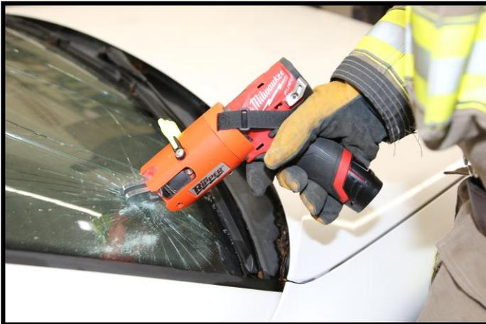
*Figure 8: Punching Starter Hole*
