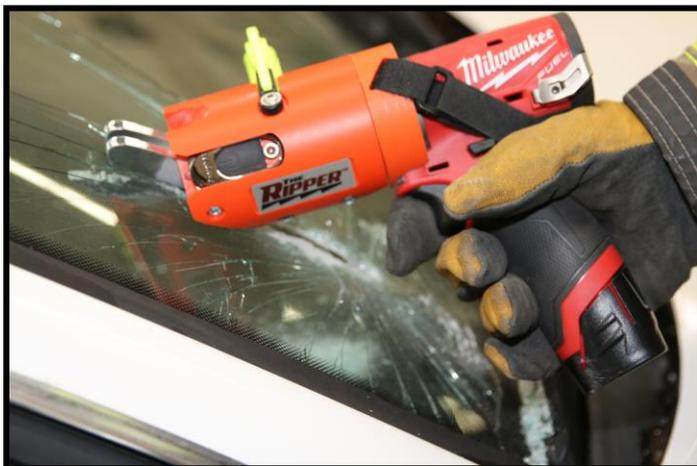
*Figure 9: Cutting Laminated Glass*
