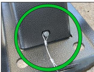
Pin must be fully inserted through the lock tab while carrying or using the Sharks™. Only remove pin during opening or collapsing of the Sharks™ and reinsert the pin prior to moving, carrying or applying load to the Sharks™. Never move or use a Shark™ without the pin fully inserted through the lock tab.
