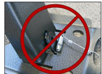
The movable Shark™ leg must be positioned outside of the lock tab. Never use an extended Shark™ with the movable leg positioned inside of the lock tab.
