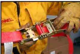
To release the strap with the drum free method, pull the trigger and rotate the handle 180° until the lock tabs can drop in the drum free slots. You may have to force the handle into this position. The drum will be free to rotate, and the strap may be pulled out. **Any load being held by the strap will be released. Use extreme caution!**
