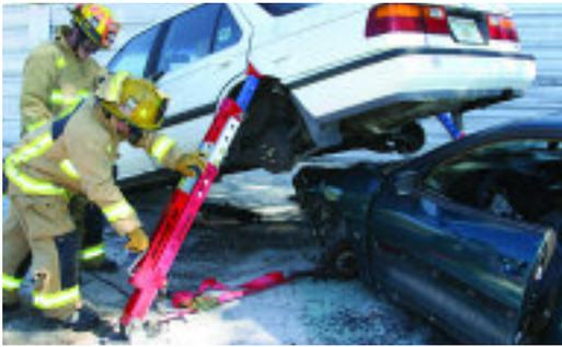
The Strut Jack is an excellent addition for lifting with the struts.
