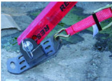
The struts from Rescue 42's TeleCrib Stabilization System are easy to put into operation. Inset: The angled portion of the base plate can take the weight.
